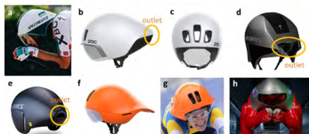
Figure 2: (a) Headsock; (b-d) Helmet with large exit opening; (e) Helmet with exit opening; (f,g) Large helmet to also guide flow over shoulders; (h) Speedski helmet. Sources: (a) https://www.specialized.com/be/en/s-works-tt-5/p/220800?color=361520-220800 ; (b, c) https://www.airparkbikero.com/news/new-poc-time-trial-helmet-has-ultimate-cooling-ability/ ; (d) https://www.specialized.com/be/en/s-works-tt-5/p/220800?color=361520-220800 ; (e) https://specialized.com.cn/products/s-works-tt-162032-1 ; (f) https://www.pocsports.com/products/tempor?variant=38096188997784 ; (g) Belga News Agency / Alamy Stock Photo. All photos reproduced with permission.
